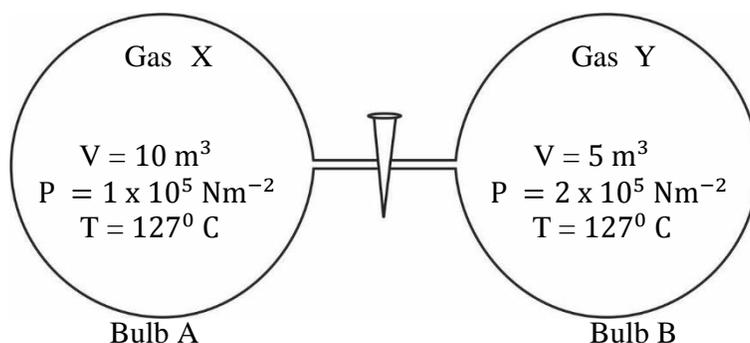
Gases were allowed to mix freely and completely by opening the tap. There is no change in the temperature of each bulb. Calculate the following in SI units assuming the ideal behaviour and the volume of the tap is negligible.
